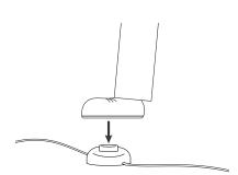
(3) Push the foot switch to turn on the lamp
