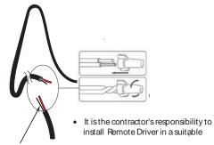
Use gel-filled waterproof wire-nuts for wire connections.
