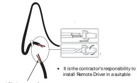
Use gel-filled waterproof wire-nuts for wire connections.
