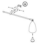
Fix the structure to the brackets 'a' and screw the bulb to the lamp holder
