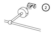
Connect the wiring with 120VAC power supply. Connect the yellow/green cable ground wire
