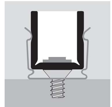
LED Strip extruded in flexible PVC and treated with polyurethane resin
