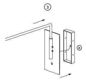
Fix the structure to the bracket 'a' and orient the stem in desired position blocking it with special screws on the cylinder
