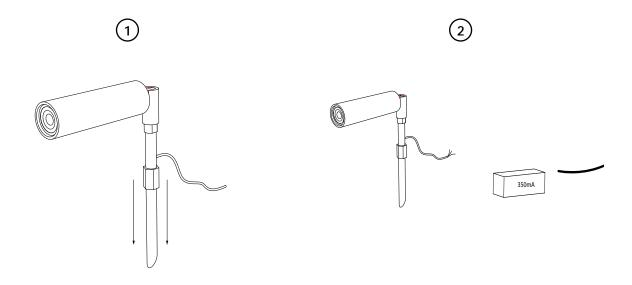
Insert the rod into the ground until the cable level with the ground
