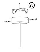
Undo the screws and fix 'c' to the ceiling
