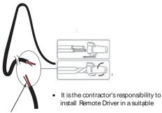
Use gel-filled waterproof wire-nuts for wire connections.
