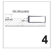
to install in remote position, minimum 11.48 feet of distance from water.
