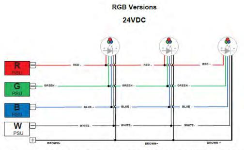
The individual lamps must be connected in parallel. Only power up the system once all the lamps have been connected.
