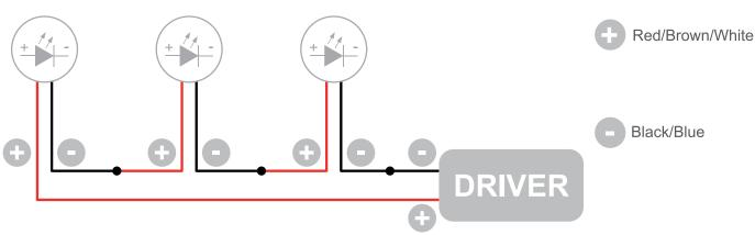
The individual lamps must be connected in series.
