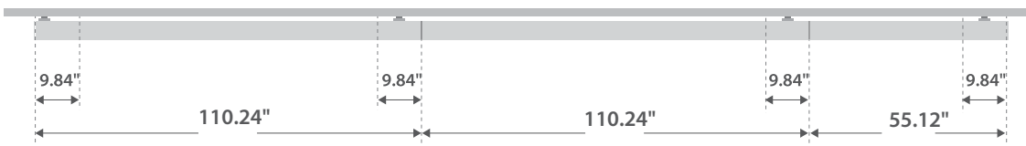
Suspended and Surface Mounted Continuous Fixing Locations
