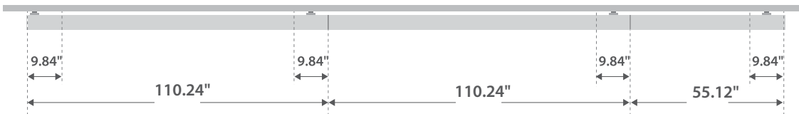
Suspended and Surface Mounted Continuous Fixing Locations
