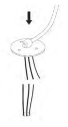
do the wiring respecting +/- polarity, heated the joints to make it watertight, connect the yellow/green ground wire
