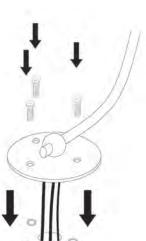
secure the plate to the around using appropriately dimensioned rawplugs. The size of rawplugs depends on the specific installation and that's the installer's responsibility.
