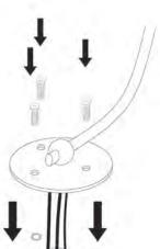
2. secure the plate to the around using appropriately dimensioned rawplugs.
