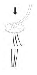
1. do the wiring respecting +/- polarity, heated the joints to make it watertight, connect the yellow/ green ground wire
