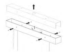
1. undo the screws and fix the bracket to the ceiling
