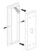
1. undo the screws and fix the bracket to the wall
