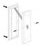
3. install 120V remote driver respecting +/- polarity, fix the structure to the bracket and tighten the side screws
