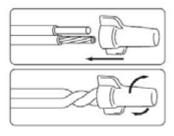
Use gel-filled waterproof wire-nuts for wire connections.
