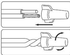
**Use gel-filled waterproof wire-nuts for wire connections.**
