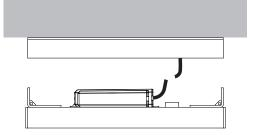
Feed the electrical cable through the central hole in the mounting bracket
