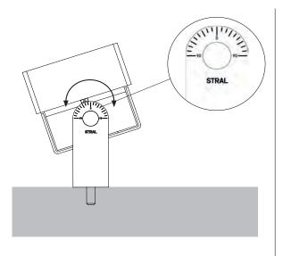
Adjust the tilt angle as desired using the graduated adjustment ring
