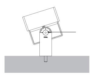
Once the desired tilt angle is set, tighten the two lateral screws to lock the projector in position
