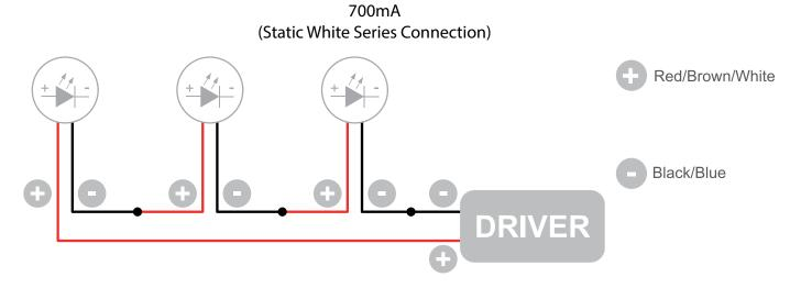
The individual lamps must be connected in series.
