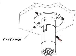
• Adjust 4 set screws to set up the designated position of fixture.
