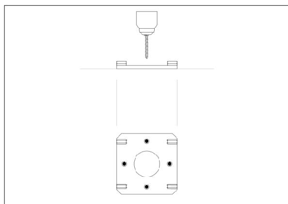
Drill at the marked points. Remove the debris.
