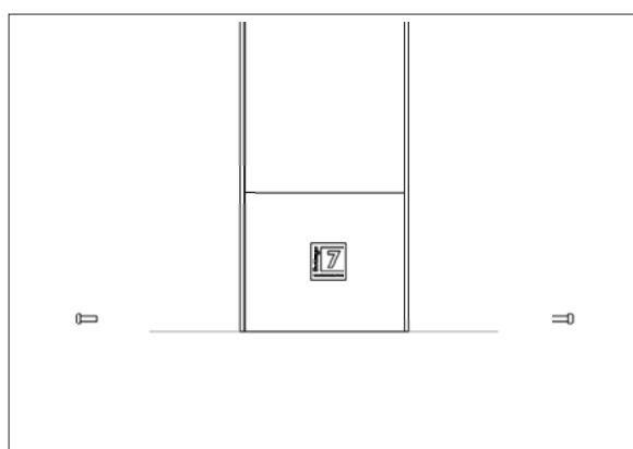
Position the bollard and fix the four screws
