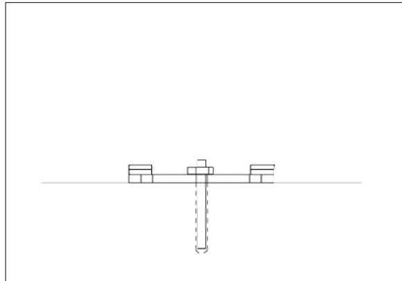
Screw the dowel in with a nut
