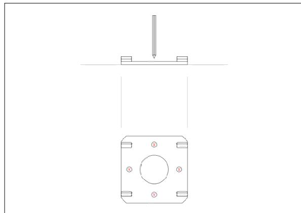
Position the template at the center of the plinth and ensure the presence of the power cable.
