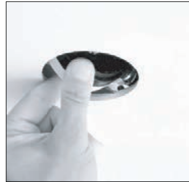
08. Detach the body from the motor magnet
