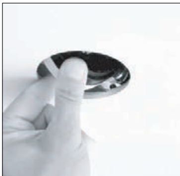
09. Push upwards until the LED module is released from the front fork and the motor magnet
